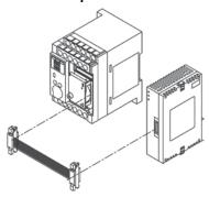
3. Push the expansion connector cable inside.
