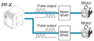
Pulse/direction and clockwise/counter -clockwise output are supported.
