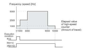
Note) When the execution condition R10 of the F174 (SP0H) instruction goes on, the high-speed counter control flag R911C (R911D) goes on. When the elapsed value reaches 10000 and pulse output stops, R911C (R911D) goes off.
