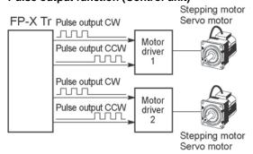
Combined with a commercially available motor driver, the function enables positioning control. With the exclusive instruction, you can perform trapezoidal control, home return, and JOG operation.
