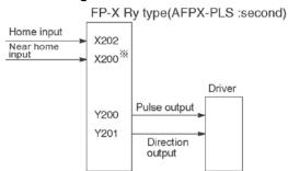
\* Input such as X200 or X201 on the pulse I/O cassette can be specified for the near home input.
