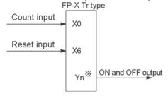
\* The output turned on and off when the target value is reached can be specified as arbitrary output of the main unit or add-on cassette.
