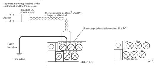
Confirm that the power supply voltage is within the allowable range of the power supply.
