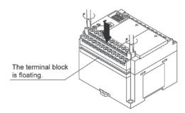
The tightening torque should be 0.25 to 0.35 Nom.
