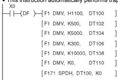
Pulses are generated from output Y0 at an initial speed of 500 Hz, a maximum speed of 5000 Hz, an acceleration/ deceleration time of 300 ms, and a movement amount of 10000 pulses.
