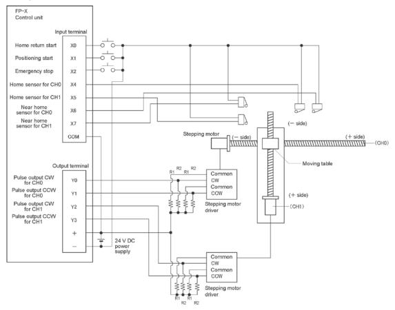
Note) When the stepping motor input is a 5 V optical coupler type, connect a 2 k $\Omega$  (1/2 W) resistor with the R1 and a 2 k $\Omega$  (1/2 W) to 470  $\Omega$  (2 W) resistor with the R2.
