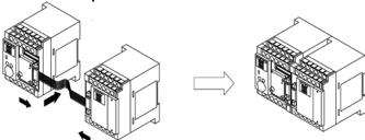
4. Set the terminator setting switch. All the switches of the expansion unit installed at the last position should be on.
