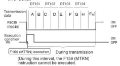
3. When all of the specified quantity of data has been transmitted, the S value is cleared to 0 and the "transmission done" flag R9039/R9049 turns on.
