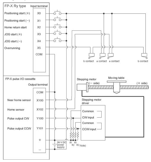
Note) When the stepping motor input is a 5 V optical coupler type, connect a 2 k $\Omega$  (1/2 W) resistor with the R1 and a 2 k $\Omega$  (1/2 W) to 470  $\Omega$  (2 W) resistor with the R2.
