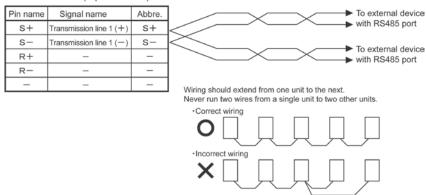
With 1:N communication, the various RS485 devices are connected using twisted pair cables. Use only one (+) and (-) terminals.
