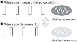
By using the exclusive instruction, the PWM output function enables a pulse output of the desired duty ratio.
