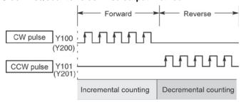
Control is carried out using two pulses: a forward rotation pulse and a reverse rotation pulse.
