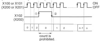
The reset input is executed by the interruption at (1) on (edge) and (2) off (edge).
