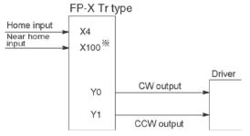
\* Input that is not used for other applications is specified for the near home input.
