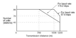
When using a baud rate of 300 bps to 38400 bps, you can set up to a maximum of 99 units (stations) and maximum transmission distance of 1200 m.
