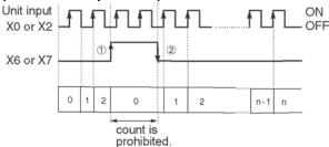
The reset input is executed by the interruption at (1) on (edge) and (2) off (edge).
