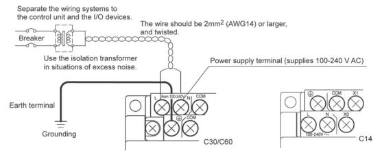
Confirm that the power supply voltage is within the allowable range of the power supply.
