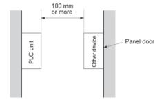
• Leave at least 100mm of space open from the front surface of the control unit in order to allow room for programming tool connections and wiring.
