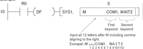
When R0 turns on, the response of COM1 port (RS485 port) delays for two scans. If the scan time is 500µs, it delays for 1 ms.
