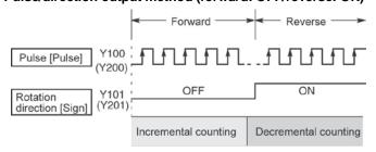
Control is carried out using one pulse output to specify the speed and another to specify the direction of rotation with on/off signals. In this mode, forward rotation is carried out when the rotation direction signal is OFF.
