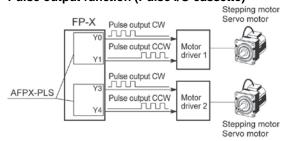
Combined with a commercially available motor driver, the function enables positioning control. With the exclusive instruction, you can perform trapezoidal control, home return, and JOG operation.
