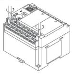
As the mounting screws are fixed at the terminal block, they are not come off even after the terminal block was removed from the main unit.
