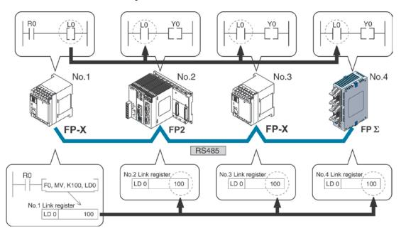
Only the COM1 port can be used for the PC(PLC) link. (Excluding AFPX-COM5)
