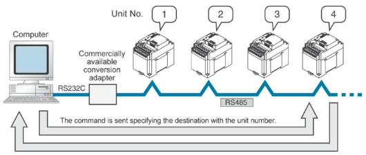
The PLC to which the response is sent is identified with the unit number.
