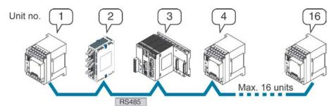
Unit numbers are the numbers to identify the different PLCs on the same network. The same number must not be used for more than one PLC on the same network.
