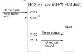
\* Input such as X100 or X101 on the pulse I/O cassette can be specified for the near home input.
