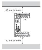
Maintain at least 100mm of space between devices to avoid adverse affects from noise and heat when installing a device or panel door to the front of the PLC unit.
