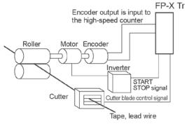
The high-speed counter function counts external inputs such as those from sensors or encoders. When the count reaches the target value, this function turns on/off the desired output.
