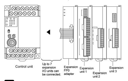
Note: Only one expansion FP0 adapter can be installed at the last position of the FP-X expansion bus. (It should be installed at the right hand side of the AFPX-E16 and E30.)
