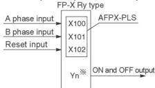
\* The output turned on and off when the target value is reached can be specified as desired from the outputs of the main unit or add-on cassette.
