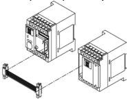
3. Push the expansion connector cable inside to touch the units each other.
