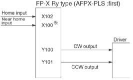
\* Input such as X100 or X101 on the pulse I/O cassette can be specified for the near home input.
