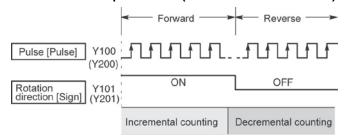
Control is carried out using one pulse output to specify the speed and another to specify the direction of rotation with on/off signals. In this mode, forward rotation is carried out when the rotation direction signal is ON.
