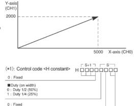
(\*2): Composite speed (Initial speed, Max. speed) (Hz) <K constant> 1.5 Hz to 100 kHz [K1 to K100000]
