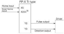
\* Input that is not used for other applications is specified for the near home input.
