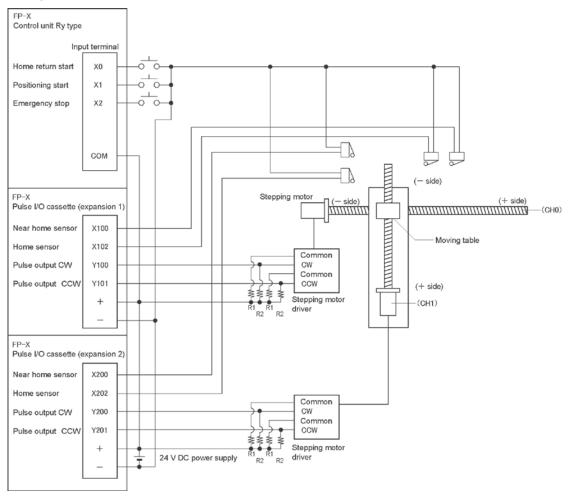
Note) When the stepping motor input is a 5 V optical coupler type, connect a 2 k $\Omega$  (1/2 W) resistor with the R1 and a 2 k $\Omega$  (1/2 W) to 470  $\Omega$  (2 W) resistor with the R2.
